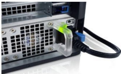
Easy troubleshooting. Functioning PSU handle glows
